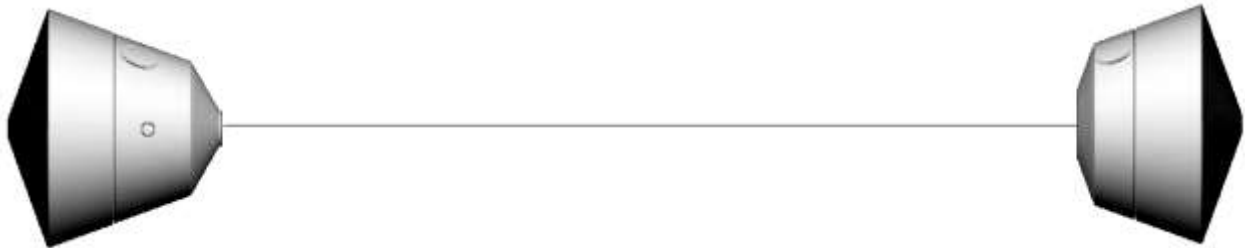
Figure 1: The two habitats are linked with a cable and rotate the one around the other to simulate the Martian gravity.
