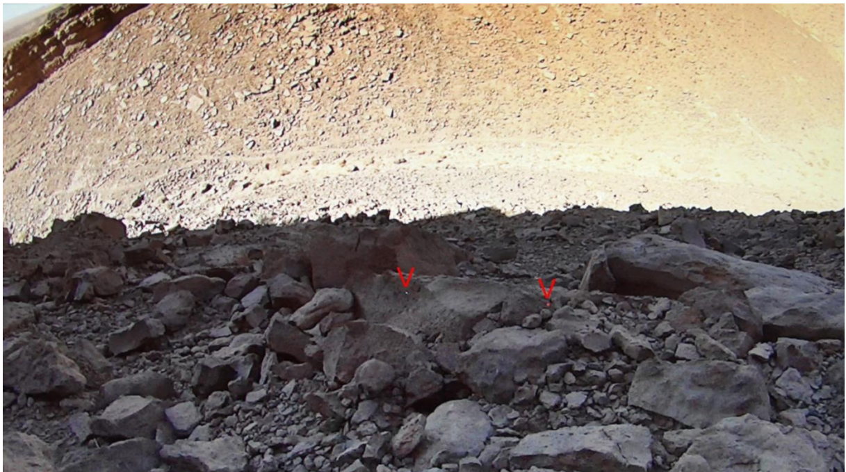
Time 6.05: “the cliffbot has landed”. The two laser spots are visible. The video shows that the vehicle has rotated by 2 \times 360^\circ + 180^\circ on the right before reaching the ground. This indicates an overhang of more than 1.3 m otherwise the antiroll rods would have stopped the rotation. The Sciencecam is now facing down slope instead of facing up slope.
